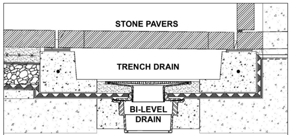
Fig. 6. Section detail at new perimeter trench drain at the LBJ Library plaza, showing a pedestal-set paver atop precast-concrete trench unit. Within the precast concrete trench, bi-level drain bodies were used.
