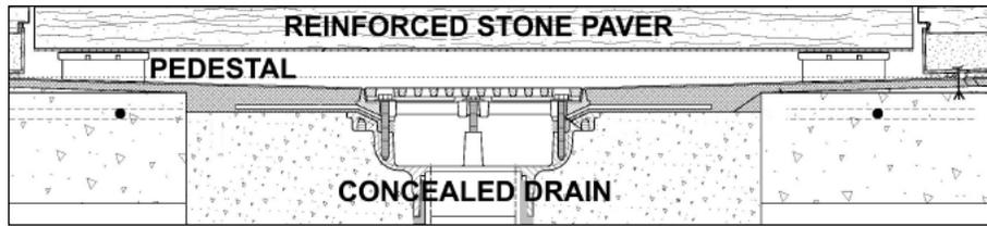
Fig. 5. Section detail at new concealed drain at the 860–880 North Lake Shore Drive plaza, showing use of pedestal-set reinforced paver. Drawing by Krueck + Sexton Architects.
