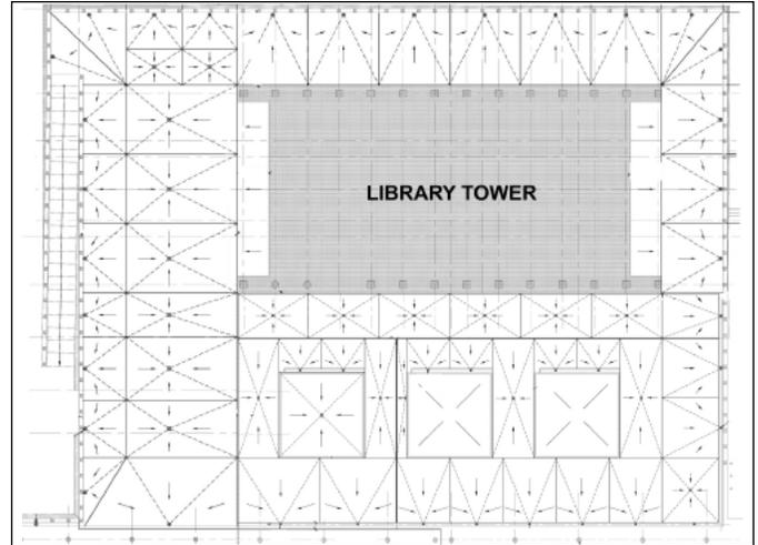
Fig. 3. Plan of the LBJ Library plaza at the subsurface (waterproofing) level, showing the slope of the new bonded overlay added atop the original structure. Each rectangular area is drained to an individual drain body.
