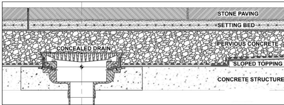
Fig. 4. General cross section of the LBJ Library plaza, showing components of the new system.
